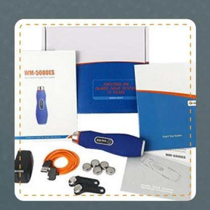
Stand alone systems can be utilised for single or multiple site applications. The data reader is downloaded to a computer via a Magnetic USB connection. Reports are generated locally. The GPP software is unlimited, so you can expand the system by adding extra Data Readers, Event Wallets or checkpoints without incurring any additional software costs.
