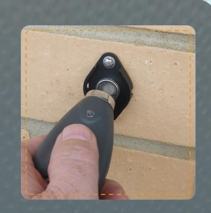
With an internal memory of 10,000 events, this small but robust reader is ideal for carrying on a lanyard or a key ring. It's also ideal for proof of presence reporting for carrying on a lanyard or a key ring. The Palm Touch does not require charging, its lithium battery has an expected life of over 12 Months or 100,000 reads
