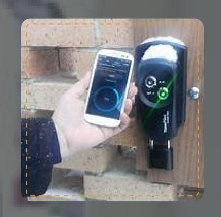
To collect the data, unlock the padlock, inserts the included USB drive into the bottom of the clock and taps a special Management iButton to one of the iButton probes.
