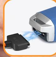
Innovative magnetic connector for improved reliability and high speed data transfer.
